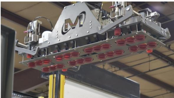
**Cold resistant B75.20 silicone cups and high-quality, powerful SX12 vacuum pumps from Piab enable flawless gripping processes.**
