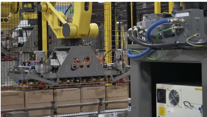
The robot picks up the cartons from a plastic belt conveyor from where the cases filled with sweet tea or juice arrive to be palletized.
