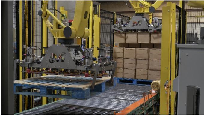
The system starts with the robot picking up a pallet and placing it onto a roller conveyor with four mechanical clamps.
