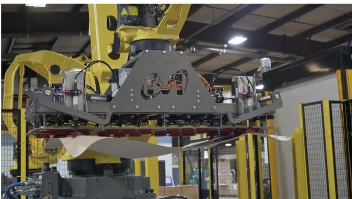
After building two layers of product the robot grabs an intermediate tier sheet and places it on the stack.
