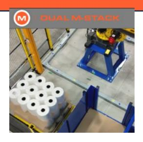
This guide highlights how the Dual M-Stack Palletizer increases throughput and reduces labor costs by enabling continuous operation. Unlike traditional systems, the Dual M-Stack supports one line-but features a key enhancement: a built-in safety door. This allows operators to remove and replace pallets on one side while the robot continues stacking on the other, eliminating costly downtime.
