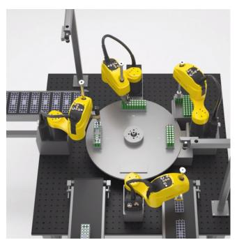
SR-3iA SCARA Robots assembling battery packs
