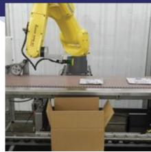
The Ergobot® case packing system includes the flexibility to park the robot while hand packing small runs of product
