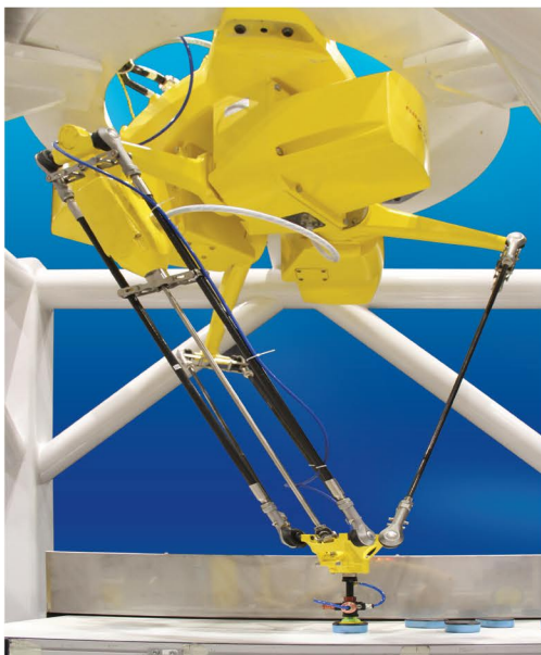
Food picking with four-axis M-2iA/3SL
