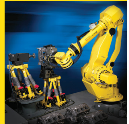
Engine block handling and deflashing with Intelligent M-900iA/350 and F-200iB robots.
