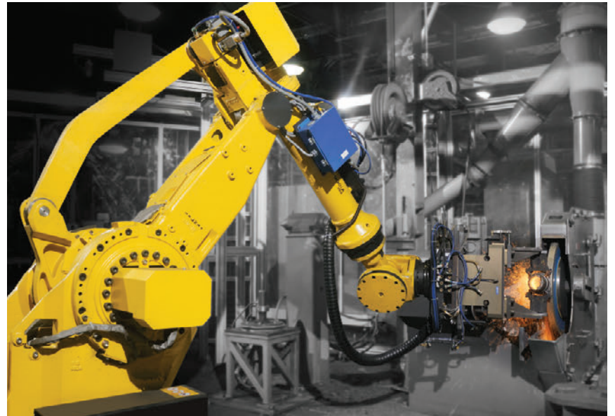
M-900 i A/350 grinding risers and heavy flash from ductile iron parts.
