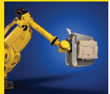
Sand core handling with M-900iA/600.
