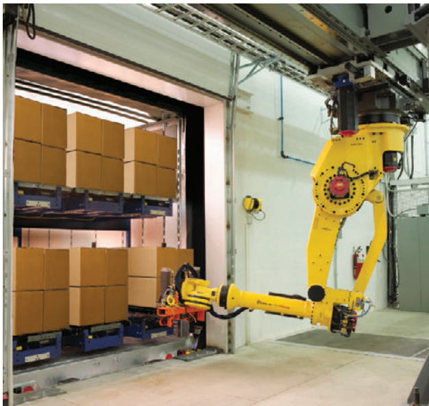
Ceiling mounted M-900 i A/350 unloading trucks.
